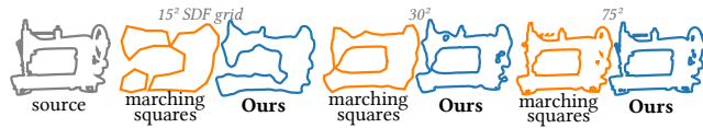
Figure 5: In 2D, our algorithm extracts significantly more geometric detail than Marching Squares on the same data.
