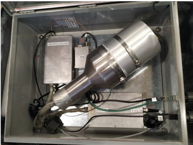
Fig. 10 X-ray sensor from the University of California, Santa Cruz working in the continuous mode
