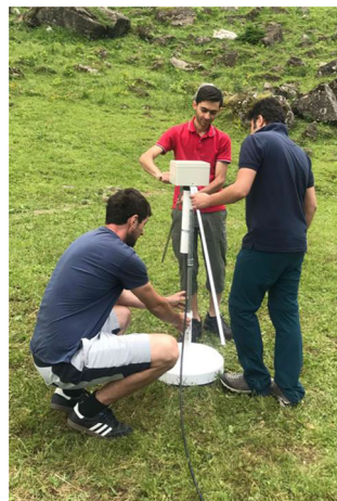
Fig. 13 Picture of personnel from the HES-SO and the EPFL installing the antennas close to the Säntis Tower for use in the 2019 measurement campaign. From left to right: Antonio Sunjerga, Amirhossein Mostajabi, and Mohammad Azadifar
