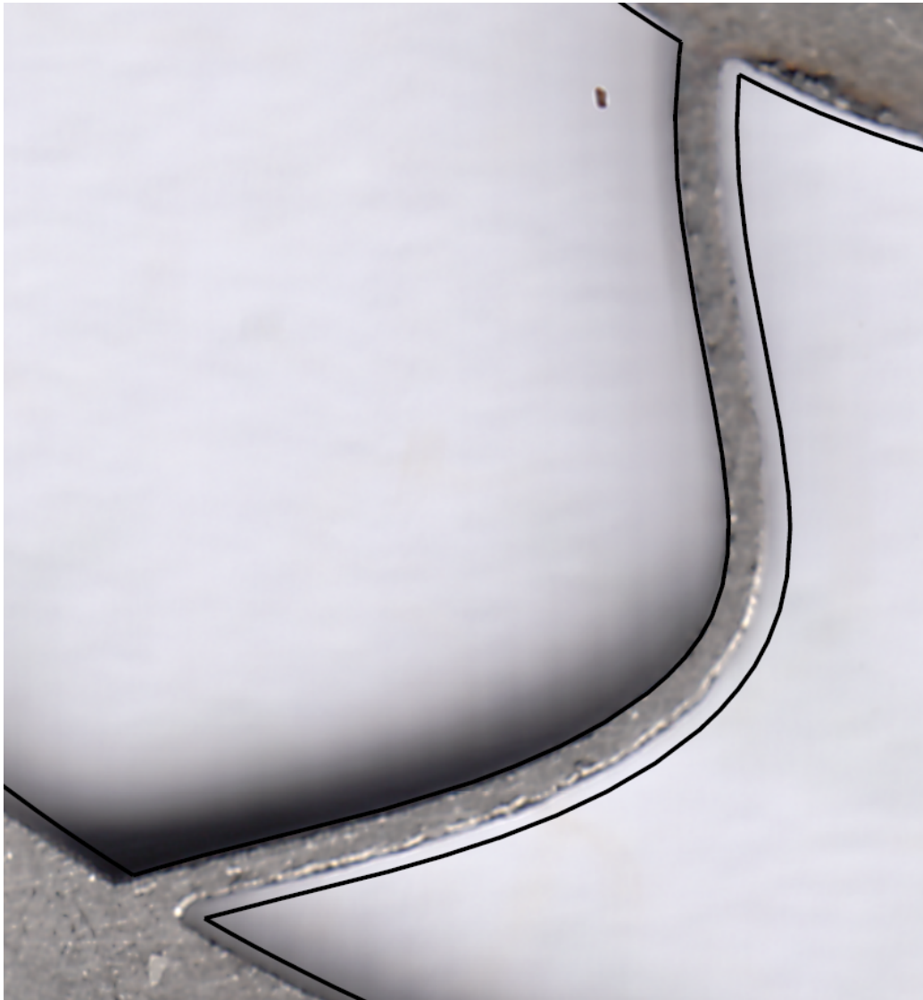
Figure 14: Overlay of designed geometry in CAD and real geometry of membrane Var23 achieved by laser cutting
