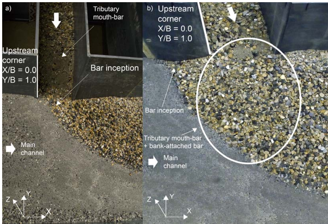
Figure 8. Upper view of the bed morphology at equilibrium for: a) \alpha = 90^\circ ; and b) \alpha = 70^\circ
