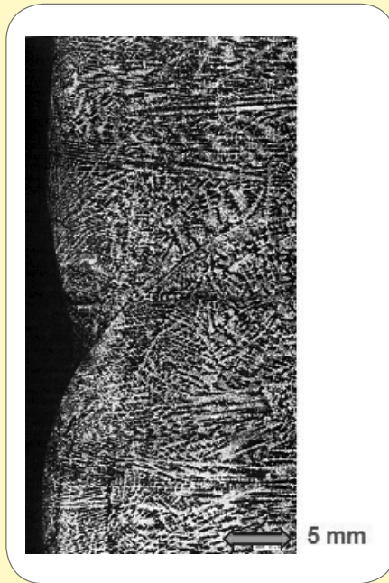
▲ Fig. 9 Hook inside a folding mark [8].
