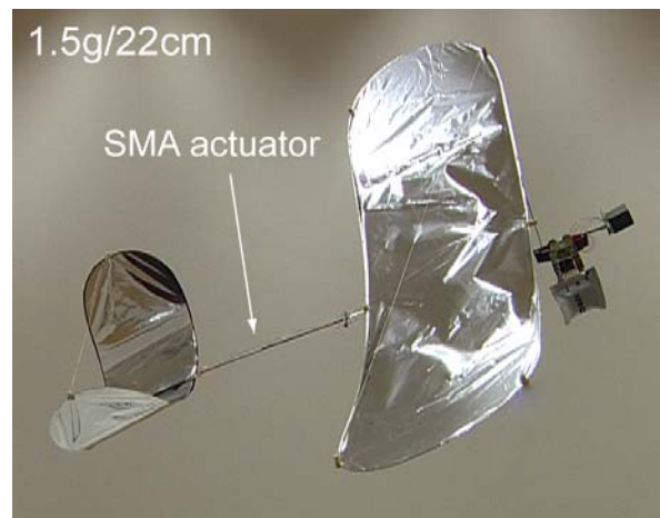
Figure 1. 1.5g Shape Memory Alloy-actuated microglider capable of autonomous phototaxis.
