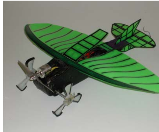
Figure 5. MALV walks on the ground using Mini- Whigs™ technology
