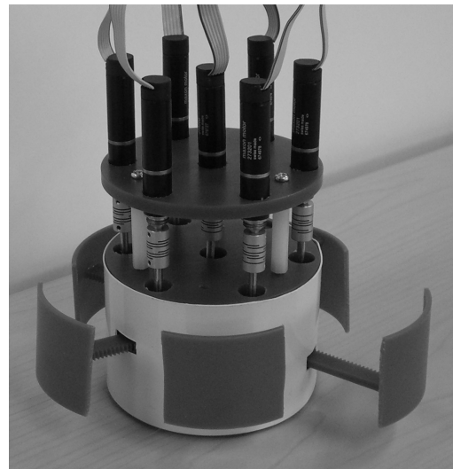
Fig. 4. A prototype of a real physical module of Slimebot.
