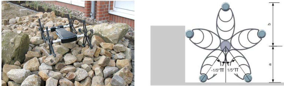
Figure 2 (left) ASGUARD in a rock channel at the DFKI outdoor test facilities, (right) the design of one ASGUARD wheel
