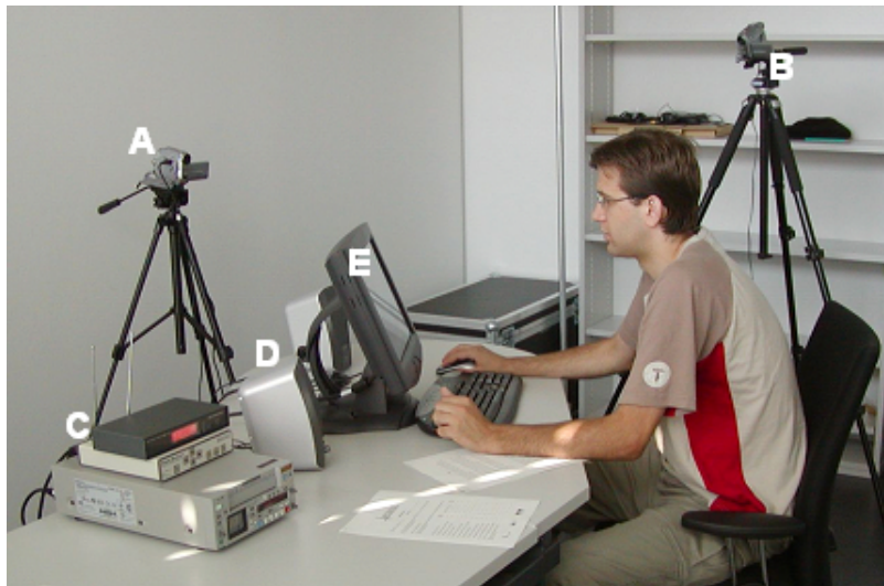
Figure 4.9: View of the user's work environment: (A) Camera that records and streams the user's face to the wizards' room (B) Camera that records the user's hands (C) Equipment for recording the user's screen (D) Loudspeakers (E) Multimodal user interface
