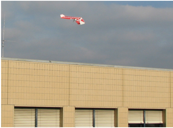
Fig. 4. The 400-gram flying wing testbed that will be used for optic-flow-based navigation in cluttered outdoor environments.
