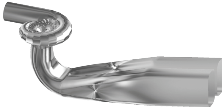
Figure 2: Computing domain of the GMS Unit 2 Francis turbine.
