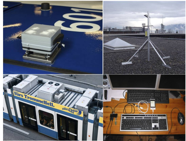
Fig. 1. Air pollution sensors that could be used in community sensing. Top left: on top of a bus; bottom left: on top of a tram; top right: attached to a solar-powered weather station on a building; and bottom right: attached to a smartphone.
