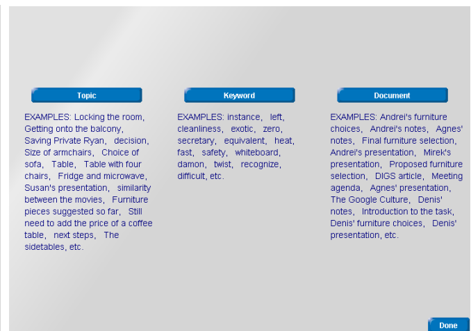
(c) Graphical component with a cue layout allowing the user to select the type of search criterion (s)he wants to specify by clicking on the corresponding button. Some examples of values for each type of specific search criterion are also displayed and the user can enter a value directly by voice or by typing it using the system's typed natural language input bar.
