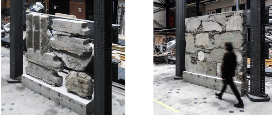
Fig. 9. Walls built out of large off-the-pile concrete rubble units ranging from 80kg to 730kg.
