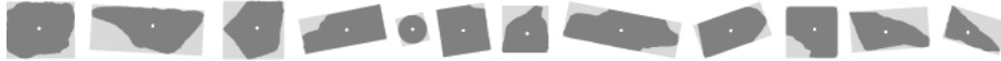
Fig. 2. Rubble pieces 2D contour geometry obtained from edge detection from top images.
