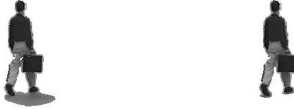
Fig. 7. Video object extraction for the test sequence Hall Monitor without (left) and with (right) shadow detection.
