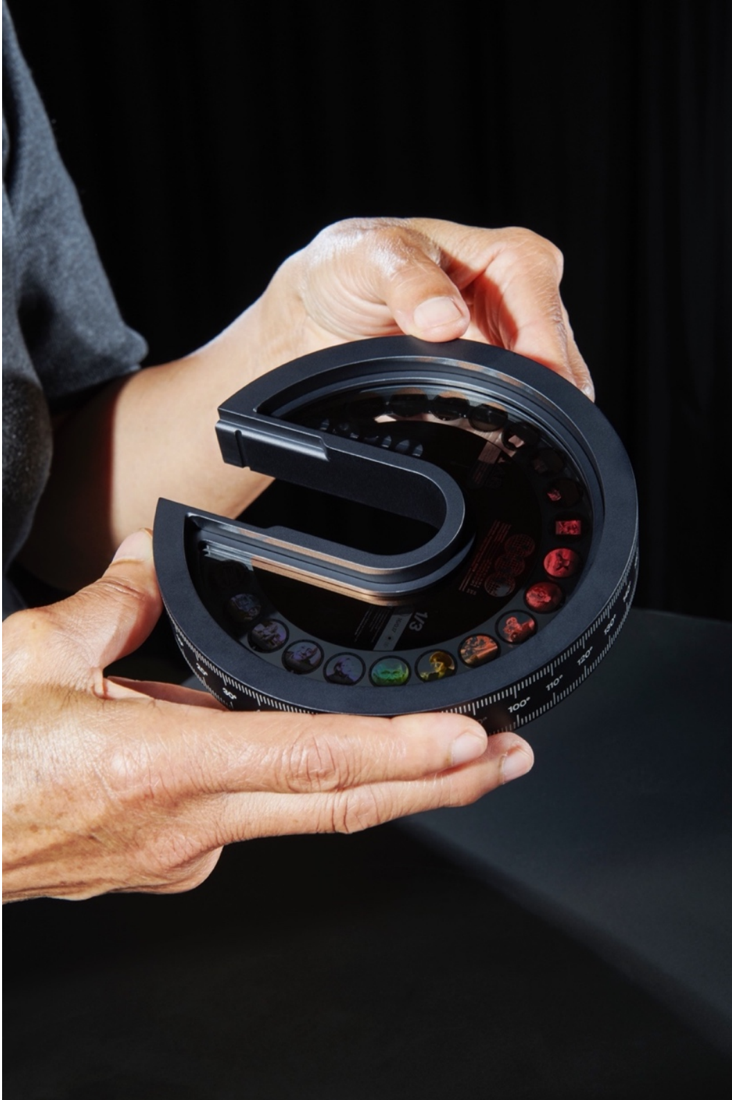
Figure 7. The summary disc of the medium-sized prototype with circular “pages” of content and the glass ball for housing synthetic-DNA in the top left of the disc. Calibration marks are engraved on the outer surface to index the content. Photography: Daniela & Tonatiuh / EPFL+ECAL Lab
