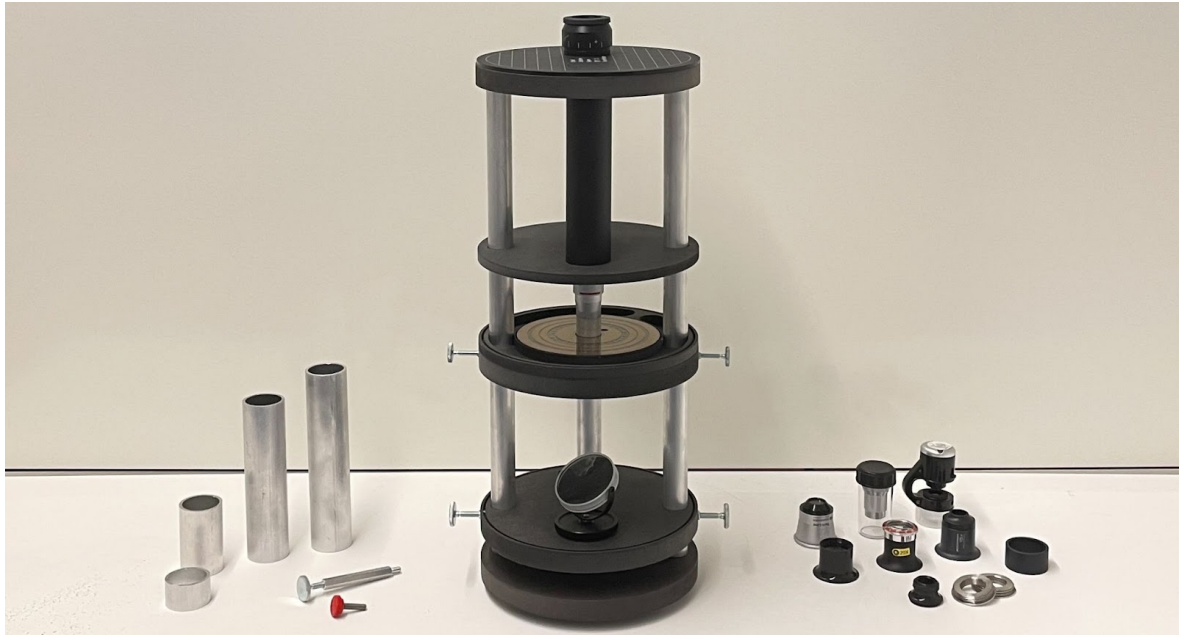
Figure 3. Tests to determine the focal length for the integrated microscope.
