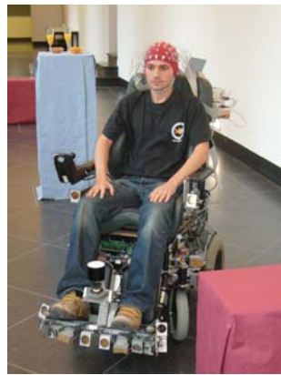
Fig. 3. Subject driving the wheelchair in a natural environment from non-invasive EEG. Note the laser scanner in front of the wheelchair, in between the subject's legs.
