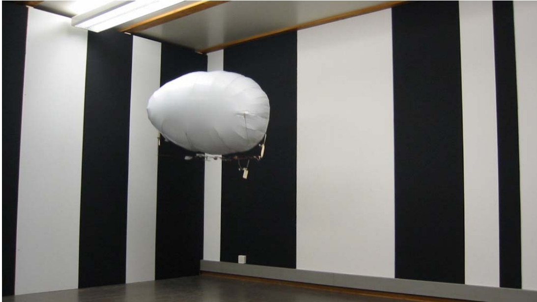
Figure 9. The evolutionary blimp in its environment, a 5 by 5 meters room with randomly spaced stripes on walls.
