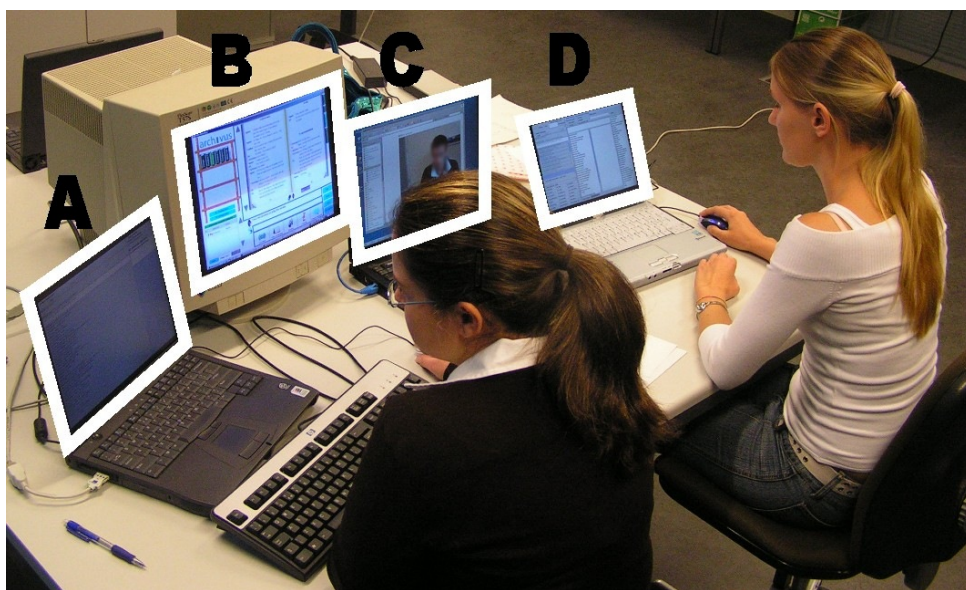
Figure 4.3: View of the wizard's environment. (A) Output Wizard's Control Interface, (B) Mirror of the user's desktop, (C) User's face, (D) Input Wizard's Control Interface.
