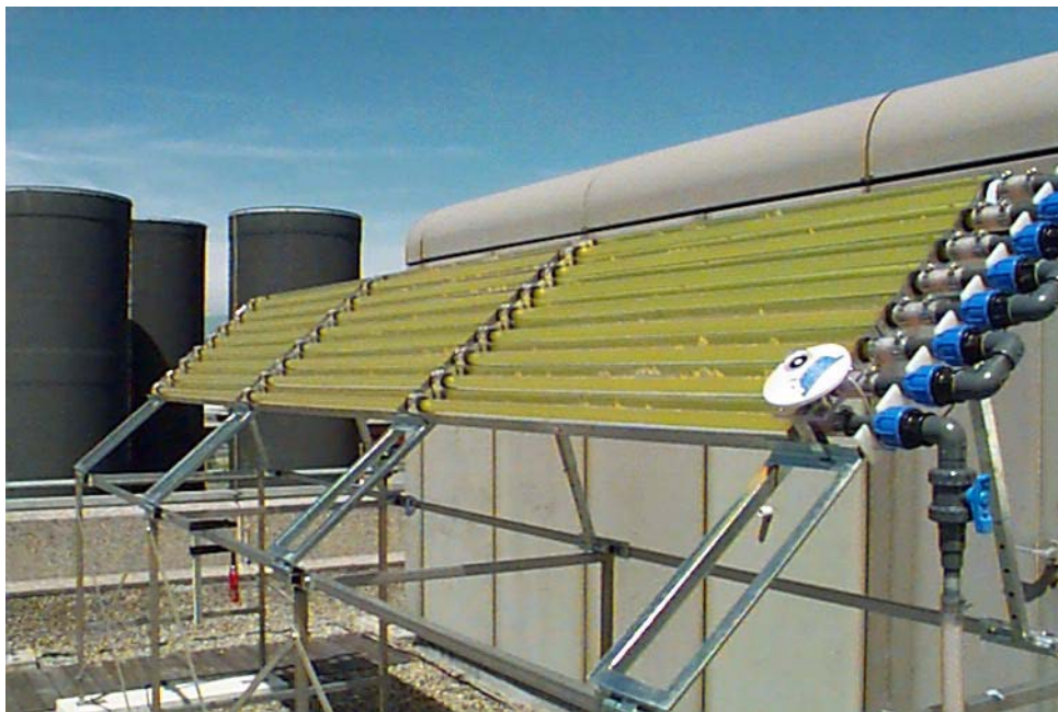
FIGURE 5.1 View of the CPC used for the solar driven experiments at the EPFL
