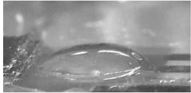
Figure 7: photograph of a 3 mm-diameter EAP actuator with 1200 V applied between the electrodes.
