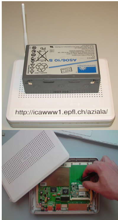
Figure 1: Illustration of the hardware used in our experimental testbed: Asus WL-500gP routers with an Atheros-based wireless card and a possible battery-based power supply.
