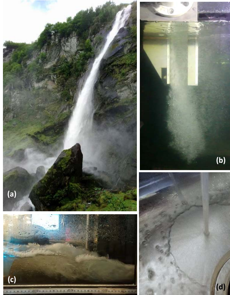
Air entrainment at (a) a waterfall, (b) a vertical supported jet, (c) a horizontal hydraulic jump and (d) a circular hydraulic jump in a kitchen sink. (Experimental flow conditions: V_1 = 4.50 m/s, Fr_1 = 13.5 , Re_1 = 5.14E+04 )
