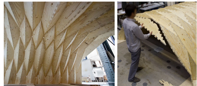
Fig. 8 The MTSJ joints have already been successfully applied to more complex assemblies, where the joint angles \theta_1 , \theta_2 and \theta_3 are not zero (Robeller et al. 2014).
