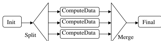
Figure 1. Flow graph describing data distribution (split), parallel processing, and collection of results (merge)
