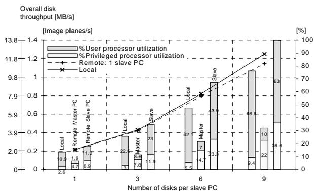
**FIGURE 10. Extracted image planes per second, overall disk throughput and processor utilization for a single processor configuration (local) and for a master - slave two processor system interconnected by Fast Ethernet (PentiumPro processors).**
