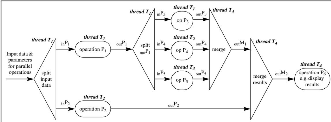
FIGURE 1. Graphical CAP macro dataflow specification
