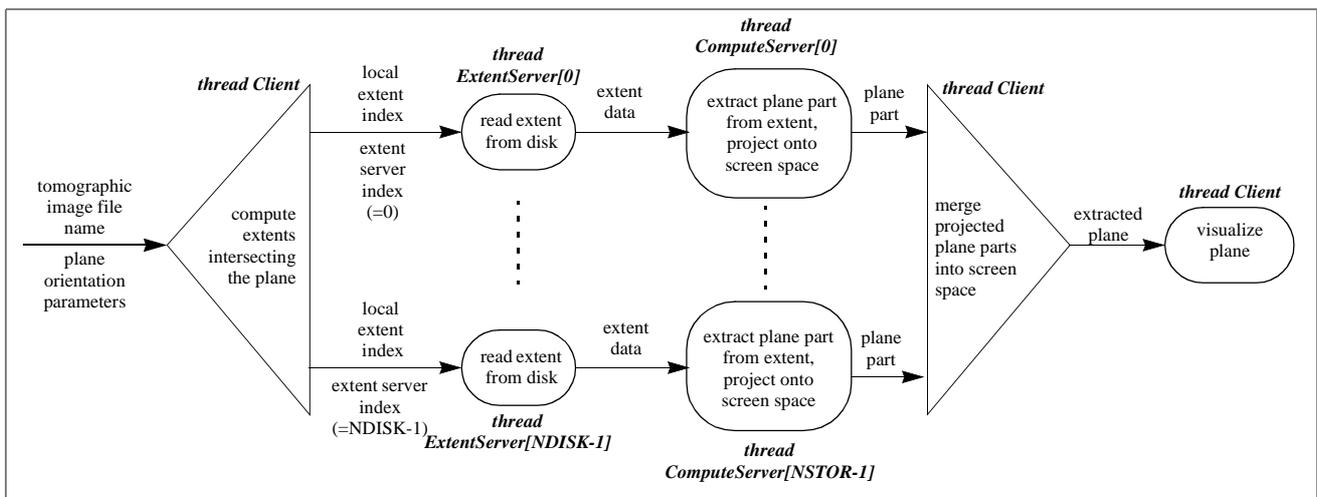
**FIGURE 7. Graphical representation of the pipelined parallel plane extraction and visualization application**
