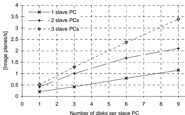
**FIGURE 11. Number of extracted image planes per second when varying both the number of disks per slave processor and the number of slave processors**
