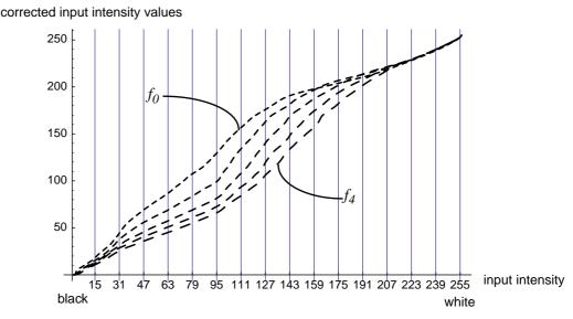
**Fig 7.** Correction tables for the 5 discrete frequencies  $f_0$ ,  $f_1$ ,  $f_2$ ,  $f_3$ , and  $f_4$ .
