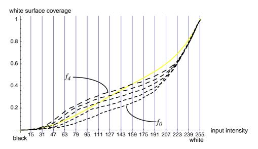
**Fig. 6.** Equivalent white surface coverage as a function of input intensity for 5 different screen element frequencies
