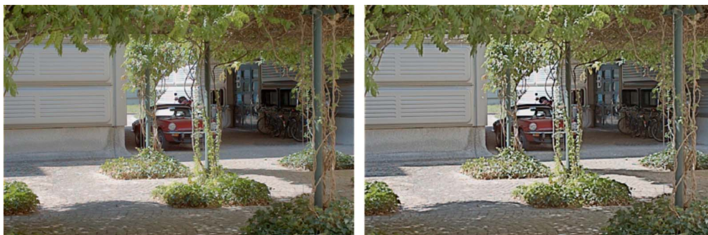
Fig. 8. (Color online) Example of our method applied with different filter sizes. Left: Small filters ( \sigma_H=1 and \sigma_A=1 ). Right: Large filter ( \sigma_H=3 and \sigma_A=5 ).
