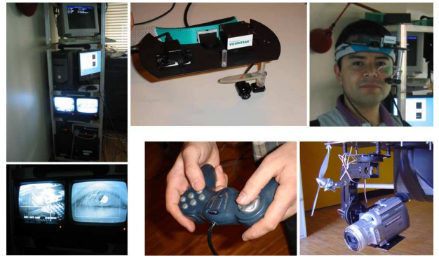
Figure 11: Top and left: The Eye-tracking system. Bottomright: The mounted rotating camera and the joystick controller.
