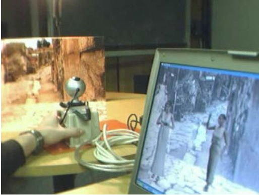
The mobile workstation with the USB webcam augmenting the real 'maquette'
