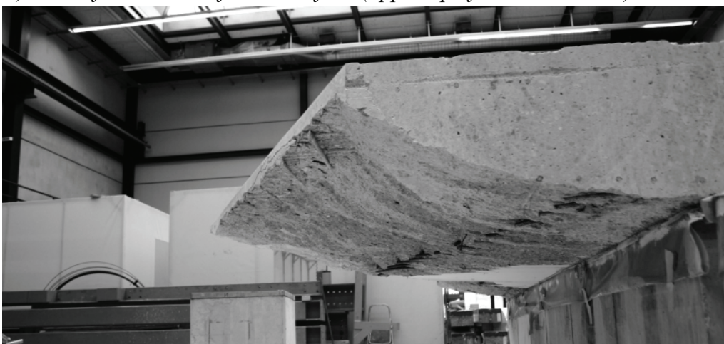
Figure A-4.20: Test DR2-a: Views of the shear crack after cutting the slab
