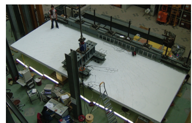
c) Test DR1-a, under four concentrated loads
