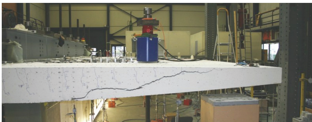
Figure A-4.35: Test DR2-c: Side view of the shear crack after failure
