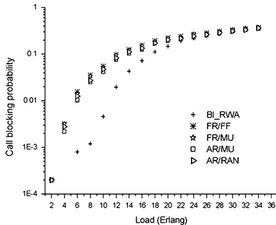
Fig. 11. Blocking probabilities for the NSFNet with four wavelengths.
