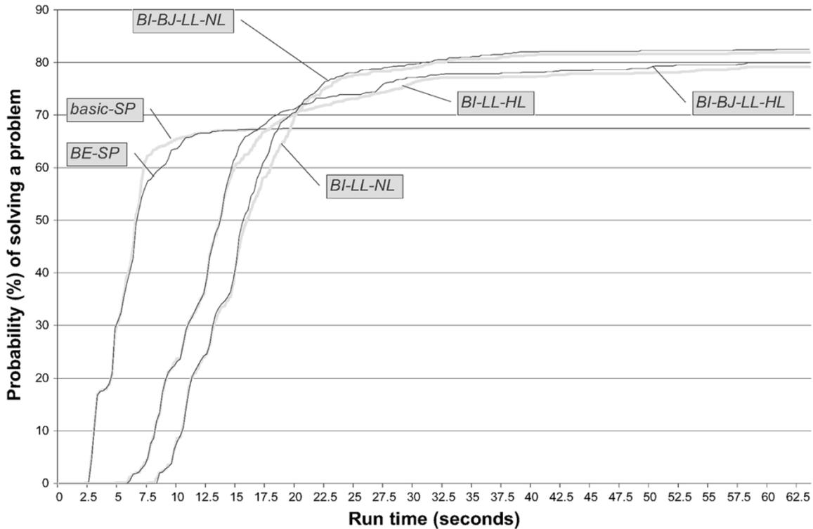
Fig. 6. Probability of solving a problem according to runtime (6000 problems, with 38 nodes, 107 links, and 1200 demands).
