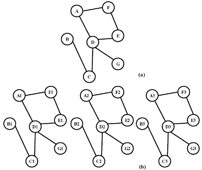
Fig. 10. (a) Network topology  $G$  with three wavelengths on each fiber link. (b) Corresponding BIGs are each composed of one BI, inside which all links have a capacity of 1.
