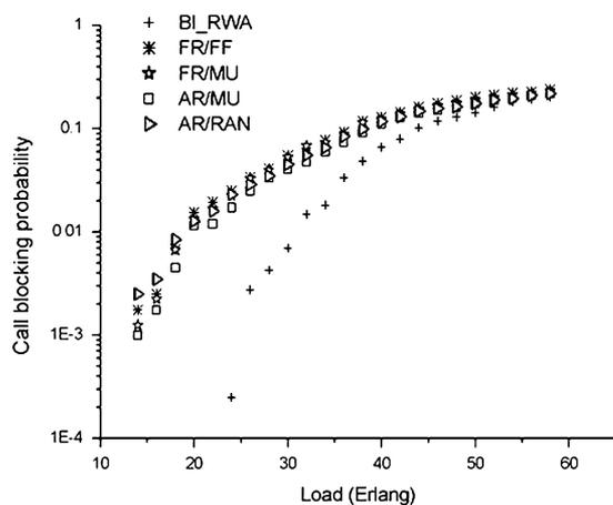
Fig. 12. Blocking probabilities for the NSFNet with eight wavelengths.
