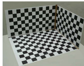
Figure 8. The sample trihedron used for the 3D reconstruction experiment.
