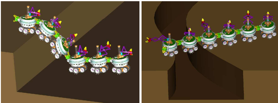
Fig. 1. Graphic visualization of how the rigid gripper can be used to connect in a secure way s-bots among themselves so to form a swarm-bot for overcoming large obstacles or holes.
