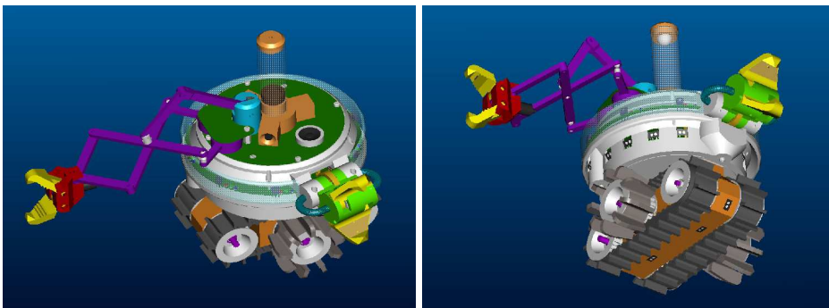
Fig. 2. Graphic visualization of the s-bot concept. The main body (turret) is equipped with passive and active gripping facilities, sensors and electronics. The lower body (traction system) is equipped with tracks and hosts the batteries. The diameter of the main body is 116 mm.
