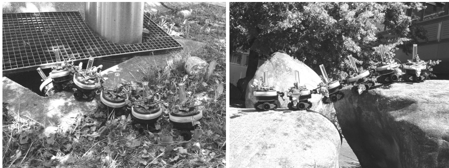
Fig. 1. A swarm-bot robot composed by six s-bots entering a building from a narrow passage (left) and passing a large gap (right).
