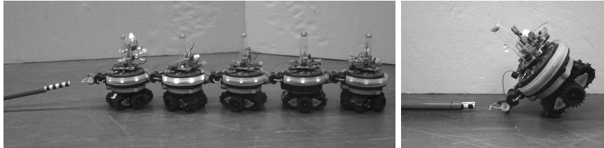
Fig. 2. Left: Chain of five s-bots forming a swarm-bot and pulling on a dynamometer. Right: One s-bot pulling the same dynamometer.
