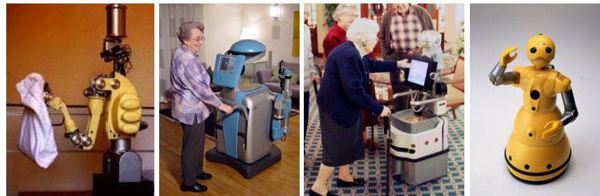
Figure 4.5. Four prototypes of assistive robots for the elderly: MOVAID, Care-O-Bot, Pearl, Wakamaru
