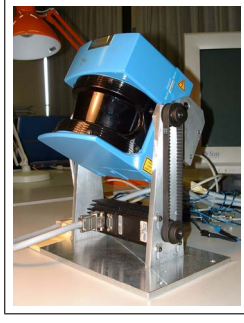
Fig. 1. The 3D sensor used is a Sick laser scanner mounted on a support which is rotated by a stepping motor via a v-ribbed belt. The angular resolution of the step motor is set to 0.45^\circ with a range of 270^\circ . The sensor produces 216961 data points (601 2D scans) per 3D scan.
