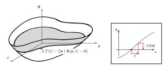
Fig. 2. In the Eulerian perspective, the wavefront is interpreted as the intersection between a graph and the zero-level of an additional dimension  $\Phi$ . The inset shows the one-dimensional case of the Eulerian formulation to clarify how equation (2) describes the wavefront's evolution: In order to make the intersection move towards the right with speed F, the whole curve  $\Phi$  has to move downwards with speed  $F|\nabla \Phi|$ .
