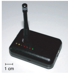
Fig. 15. Wireless base board
