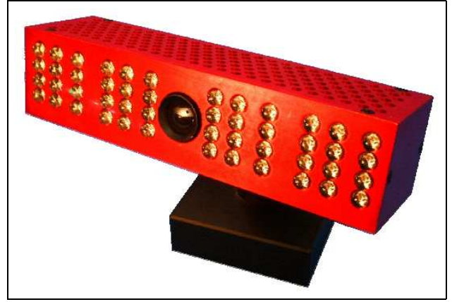
Fig. 2. The time-of-flight Swiss Ranger sensor from CSEM. Note that sensor contains no moving parts.
