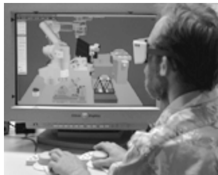
Figure 4. Two handed VR-interface using space mouse and data glove (space-station scenario as example).
