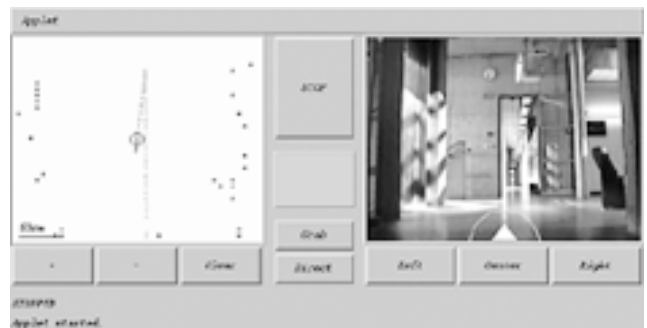
Figure 5. WebDriver enables safeguarded vehicle teleoperation via the www.
