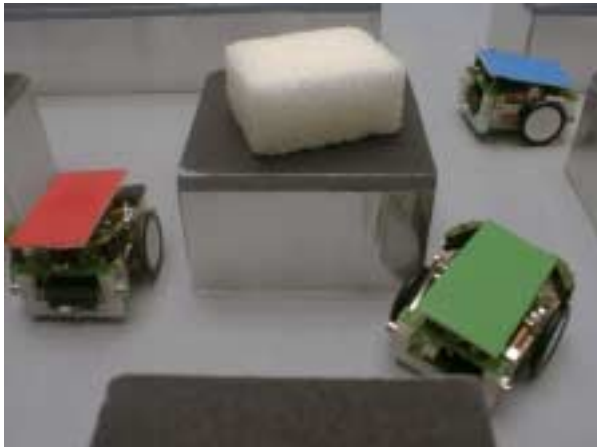
Figure 1: 3 mobile micro-robots Alice in a labyrinth. The robots and the sugar cube have the same size!
