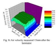
The compressed and filtered air passes through a 30 mm thickness laminator and becomes laminar. Fig. 8 shows that the air velocity measured at a distance of 15mm from the laminator is
