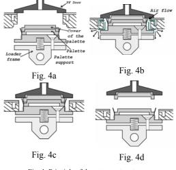
Fig. 4: Principle of the entry port system
