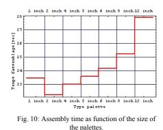
size of the palette (here in inches) to the assembly time for a given component.
