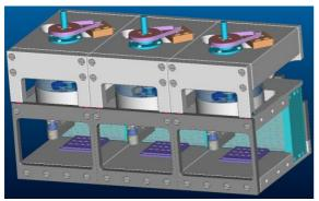
Fig. 2: A Pocket-Factory with three modules of microboxes
