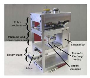
Fig. 3: The microbox is a module of the Pocket-Factory The next sections explain the functionality of these parts.
