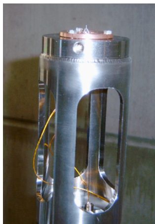
Figure 5.20: Photo of the ZrC single-tip thermionic emitter used for electron bombardment of the anode. The ZrC tip can be seen at the top clamped between two molybdenum holders. The leads connect the molybdenum holders to the BNC feedthrough at the end of the cathode cone.
