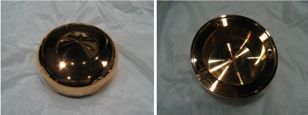
Figure 4.6: The gold plated anode electrode as seen from front (left) and back (right). The back side shows the insert for electrical isolation and solenoid magnet casing. The hole at the center is the anode beam channel downstream of the iris.
