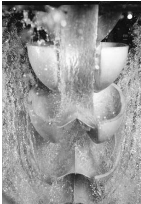
Figure 2.1: External stroboscopic flow visualization (Courtesy of VATEch Hydro SA).
