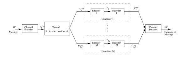
Fig. 8. The Quantized Channel Problem.
