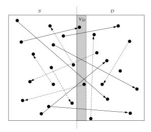
Fig. 6. The cut-set considered in the proof of Theorem 5.2. The communication requests that pass across the cut from left to right are depicted in bold lines.
