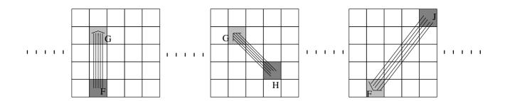
Fig. 2. Successive MIMO transmissions are performed between clusters. The first figure depicts MIMO transmission from cluster F to G, where bits originally belonging to  $s_1$  are simultaneously transmitted by all nodes in F to all nodes in G. The second MIMO transmission is from H to G, while now bits of source node  $s_2$  are transmitted by nodes in H to nodes in G. The third picture illustrates MIMO transmission from cluster F to F.
