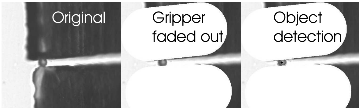
Figure 3.45: Combined gripper-object detection while the object is gripped.
