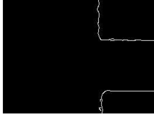
Figure 3.37: Two-jaw gripper after Canny edge detection.
