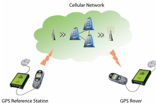
Figure 2: Direct cellular connection for GPS-RTK.
