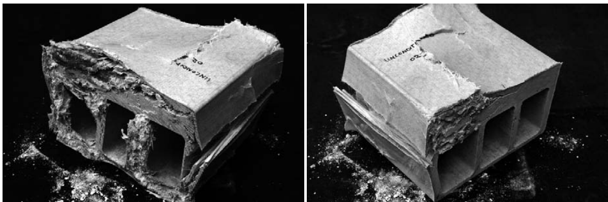
(a) Severe asymmetric crushing
