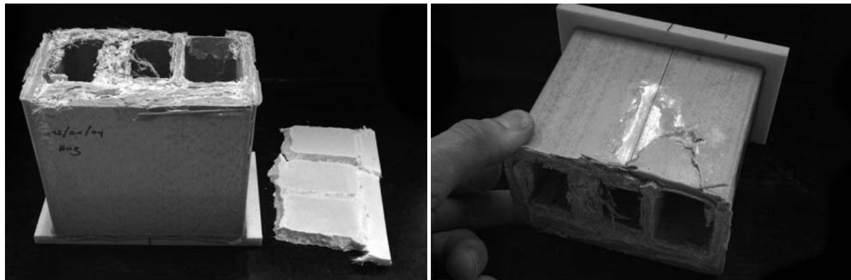
(a) Even crushing of profile end
