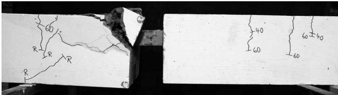
Figure G.26: Crack pattern for M3E2
