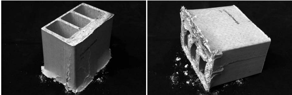
(a) Longitudinal crack on outer web
