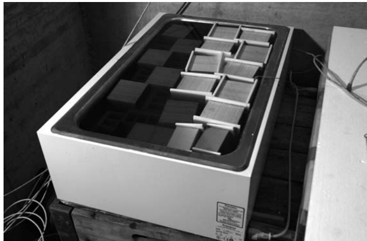
Figure 3.7: Heated bath with inserted CS-elements before covering
