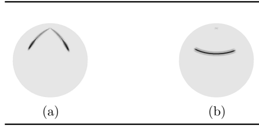
FIGURE 6 Analysis of a triangle with the spherical Morlet wavelet, in two different orientations: (a) \chi = 0^\circ ; (b) \chi = 90^\circ , showing the directional selectivity of the wavelet.
