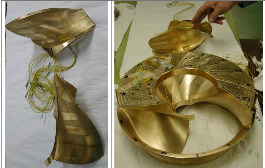
Figure 6: Views of the instrumented runner during its mounting
