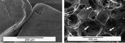
Fig. 2. Secondary electron SEM images of (a) the contact point between particles of 400  $\mu$ m NaCl after CIP at 28 MPa, and (b) the resulting foam after infiltration under 4 bar pressure ( $V_{\rm f} = 0.2$ ), with replicated cracks indicated by the white arrows.
