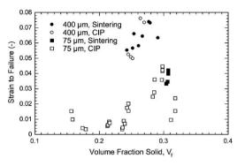
Fig. 6. Tensile elongation of foams made using preforms densified by sintering and CIP.
