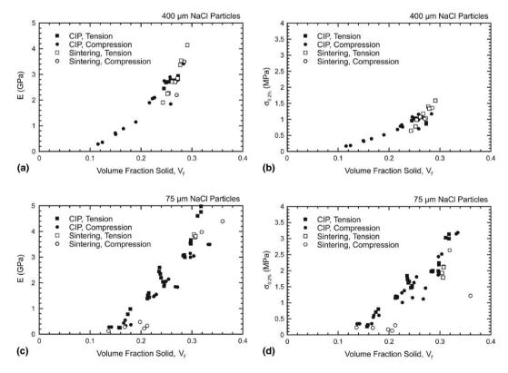
Fig. 4. The Young's modulus (graphs (a) and (c)) and 0.2% yield stress (graphs (b) and (d)) of pure aluminium foams made using preforms densified using sintering or CIP from 400  $\mu$ m (graphs (a) and (b)) and 75  $\mu$ m (graphs (c) and (d)) diameter NaCl particles, tested in tension and compression. Estimated error in testing and data analysis procedures is around 2% of the measured value; hence it roughly corresponds to the size of the points on the curves.
