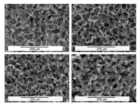
Fig. 3. Secondary electron SEM images of pure aluminium foams made by the replication method using preforms of 75  $\mu$ m NaCl particles: (a) unsintered ( $V_f = 0.4$ ), and sintered at 755 °C for (b) 2 h ( $V_f = 0.37$ ), (c) 9 h ( $V_f = 0.32$ ) and (d) 25 h ( $V_f = 0.25$ ).
