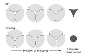
Fig. 5. A schematic diagram of three particles, showing a cross-section through the plane containing their centres, during sintering and CIP, illustrating the difference in the foam strut shapes produced.
