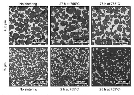
Fig. 1. Optical micrographs of polished sections through resin-infiltrated preforms of NaCl of 400  $\mu$ m and 75  $\mu$ m diameter, made by sintering at 755 °C for different periods of time. The dark phase is NaCl and the light phase is mounting resin.
